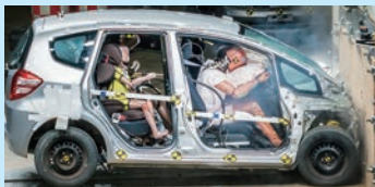
Occupant protection test for head-on collisions
