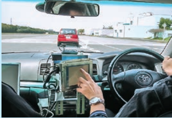
Experiment to evaluate the effect of the operation of information systems (car navigation, smart phones, etc.) on driving
