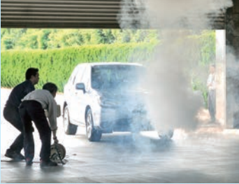
Experiment of unnecessary operation of the collision damage reduction brake
